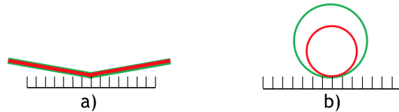
Figure C.15: Cartoon comparing the propagation directions of the red and THz pulses (colored green) grazing off the surface of gold reflective gratings with a) THz-red propagating (left to right) perpendicular ( \perp ) to the grooves and b) THz-red propagating (into the page) parallel ( \parallel ) to the grooves.
